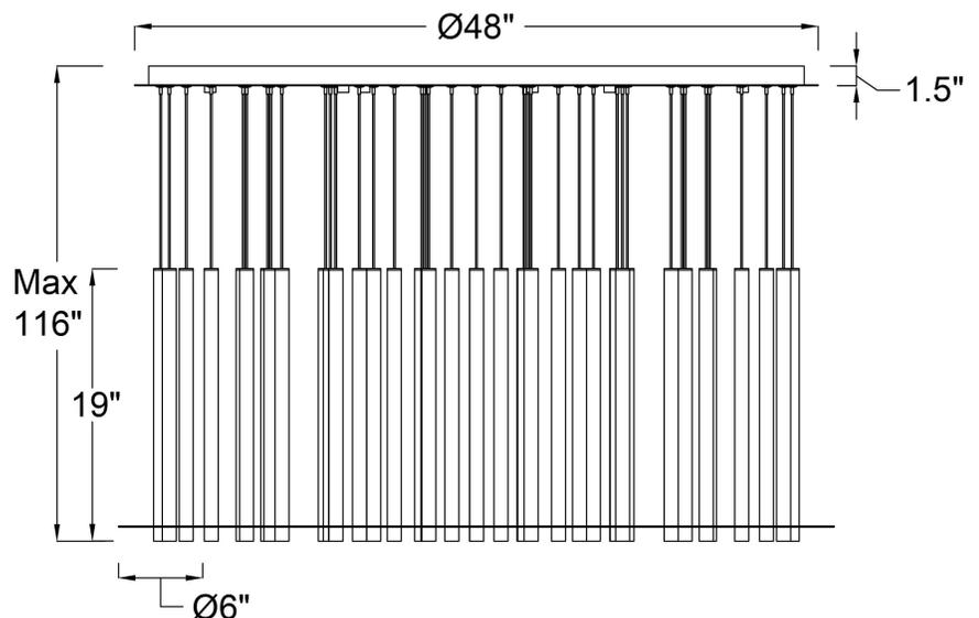
Fixtures weighing 35lbs. or more must be supported and installed independently of the ceiling outlet (junction) box and require additional support in the ceiling where the fixture is being installed.
